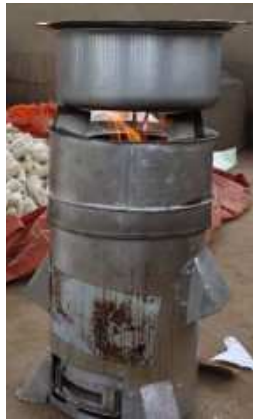
FIGURE 9 - Top Lit Updraft stove (MWOTO stove – Uganda)
