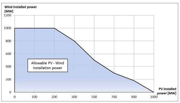
Figure 1 – Theoretical example of the allowable area on the PV/Wind installed power chart
