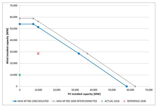
Figure 7 - VRES installed capacity limits due to system operation constraints in Brazil – 2030
