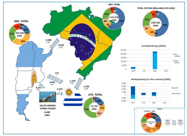
Figure 24 - Total production and energy exchanges – scenario V1a
