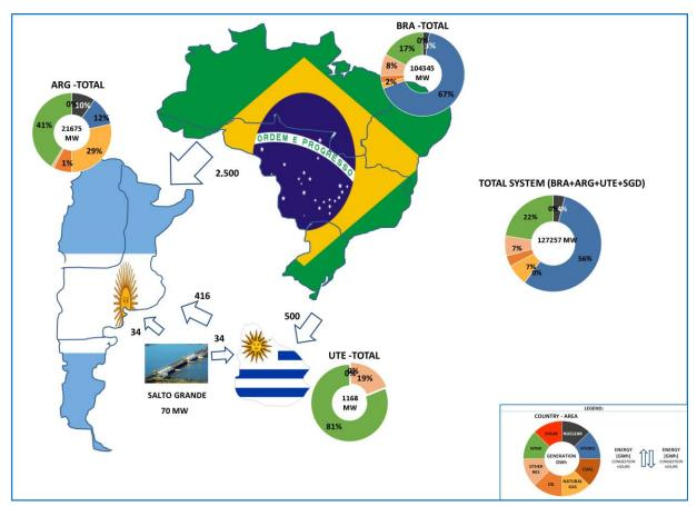
Figure 32 - Static Analysis - Power production and power exchanges in low load and low RES production
