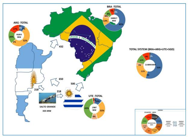
Figure 29 - Static Analysis - Power production and power exchanges with high load and high RES production
