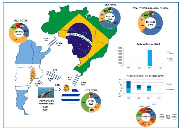
Figure 26 - Total production and energy exchanges – Reference scenario for Variant 2
