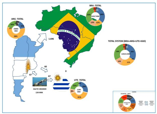
Figure 31 - Static Analysis - Power production and power exchanges with low load and high RES production
