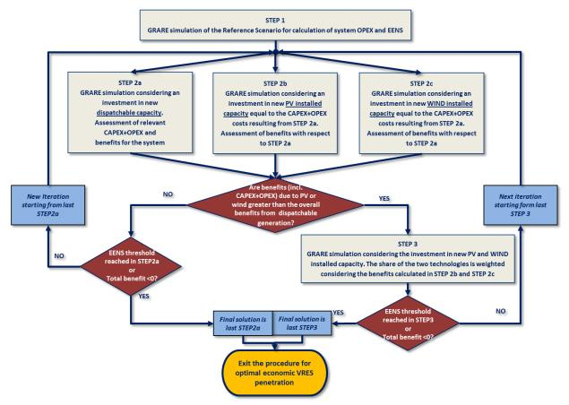
Figure 9 - Procedure for the calculation of the optimal economic VRES penetration
