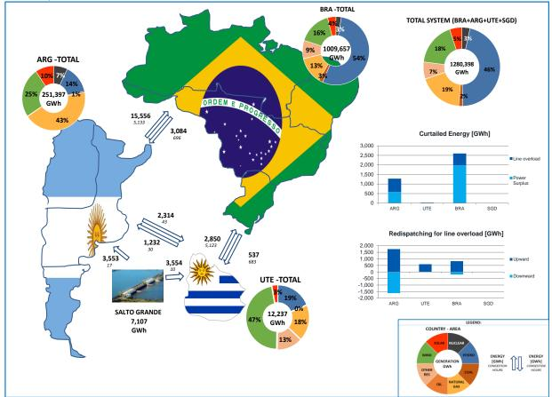
Figure 21 - Total production and energy exchanges – ARG, BRA and UY interconnected with dry hydrological conditions
