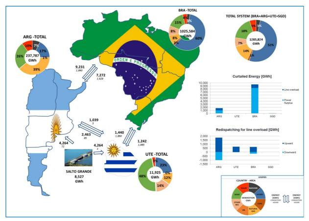
Figure 18 - Total production and energy exchanges – ARG, BRA and UY interconnected final optimal scenario
