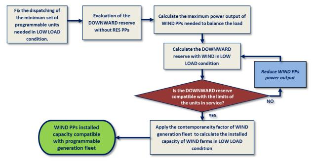
Figure 2 - iterative calculation of max installation of wind power plants
