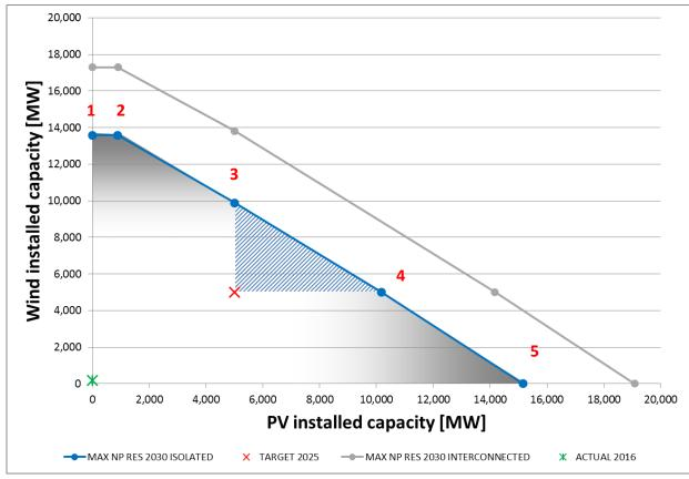
Figure 6 - VRES installed capacity limits due to system operation constraints in Argentina – 2030
