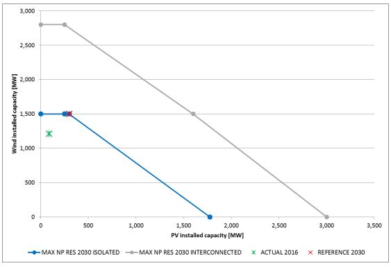
Figure 8 - VRES installed capacity limits due to system operation constraints in Uruguay - 2030
