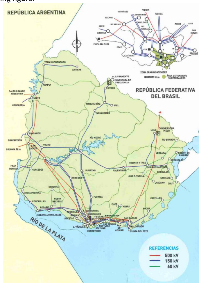
Figure 43 – Current transmission network in Uruguay [source: UTE [9]]
