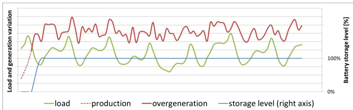
Figure 74 - Energy storage limit in case of long lasting overgeneration
