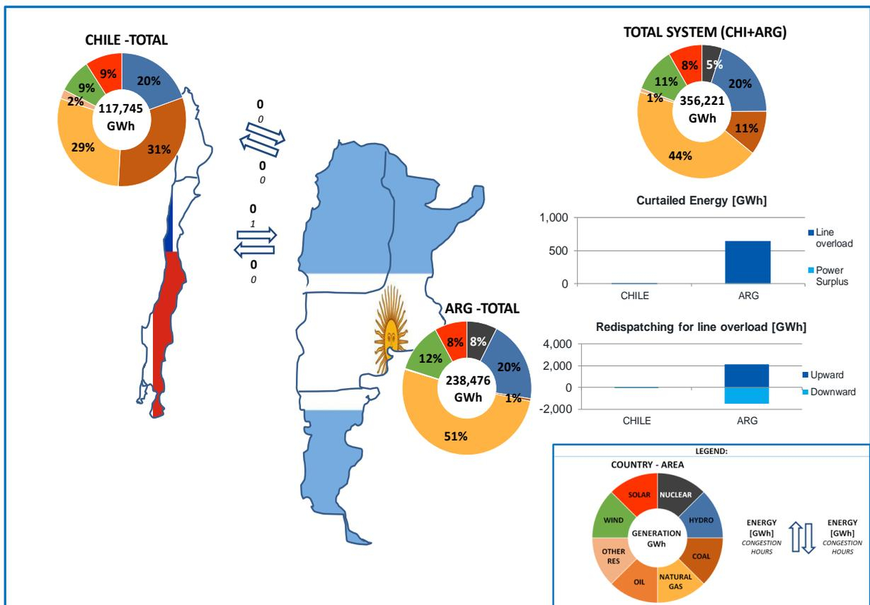
Figure 59 - Total production and energy exchanges – Reference scenario interconnected countries without energy exchanges
