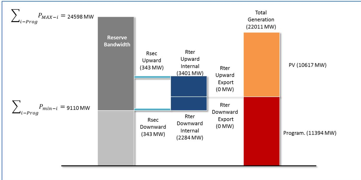
Figure 20 - Generation and reserve in Argentina - Low load and high VRES scenario, maximum PV installed capacity, no cross-border exchanges
