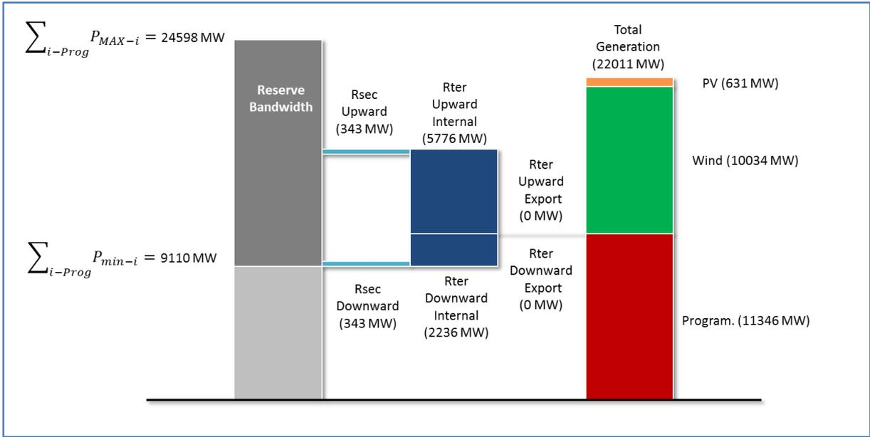
Figure 8 - Generation and reserve in Argentina- Low load and high VRES scenario, maximum wind installed capacity, no cross-border exchanges
