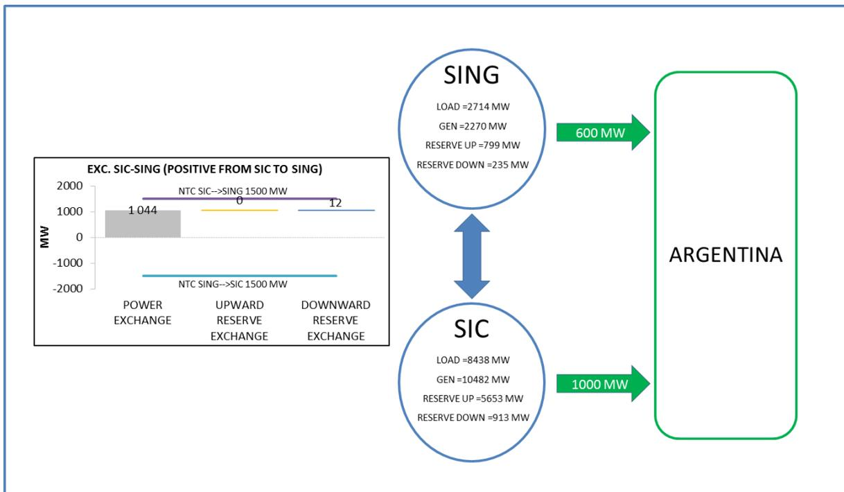
Figure 33 - Power and reserve exchanges between Chilean areas - Low load and high VRES scenario, maximum wind installed capacity meeting PV target, maximum export
