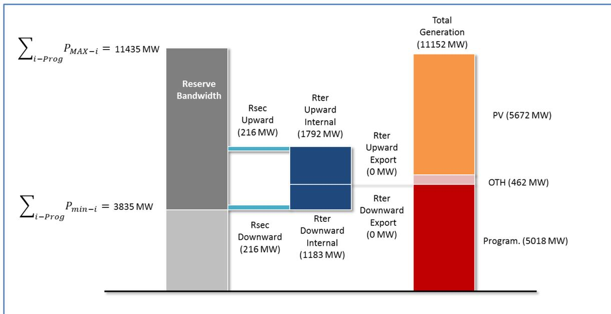
Figure 38 - Generation and reserve in Chile - Low load and high VRES scenario, maximum PV installed capacity, no cross-border exchanges
