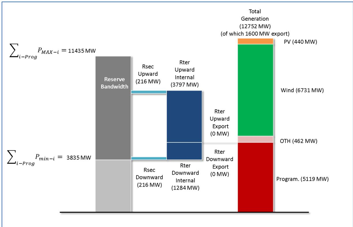
Figure 28 - Generation and reserve in Chile - Low load and high VRES scenario, maximum wind installed capacity, maximum export
