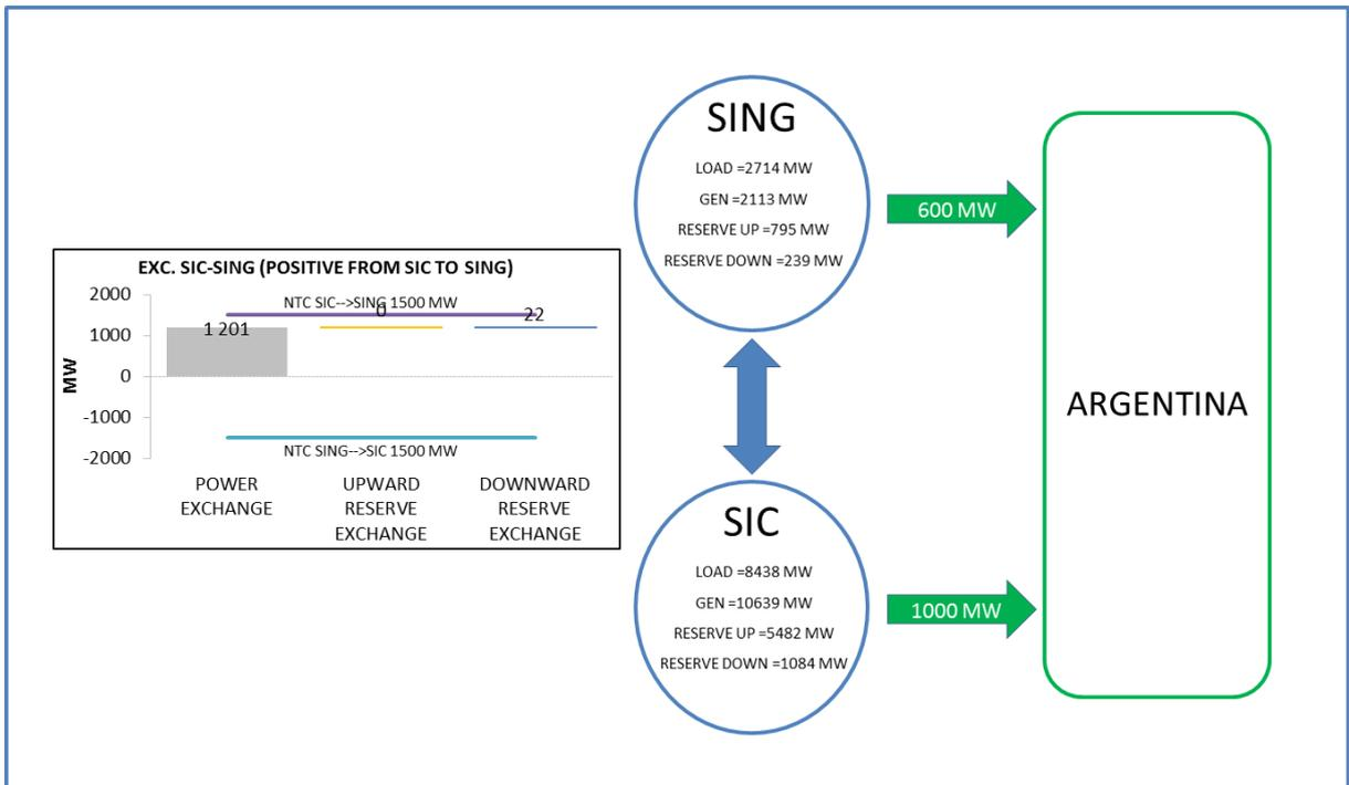
Figure 41 - Power and reserve exchanges between Chilean areas - Low load and high VRES scenario, maximum PV installed capacity, maximum export
