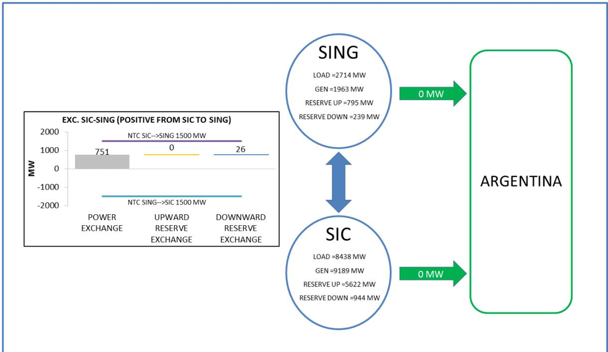
Figure 39 - Power and reserve exchanges between Chilean areas - Low load and high VRES scenario, maximum PV installed capacity, no cross-border exchanges
