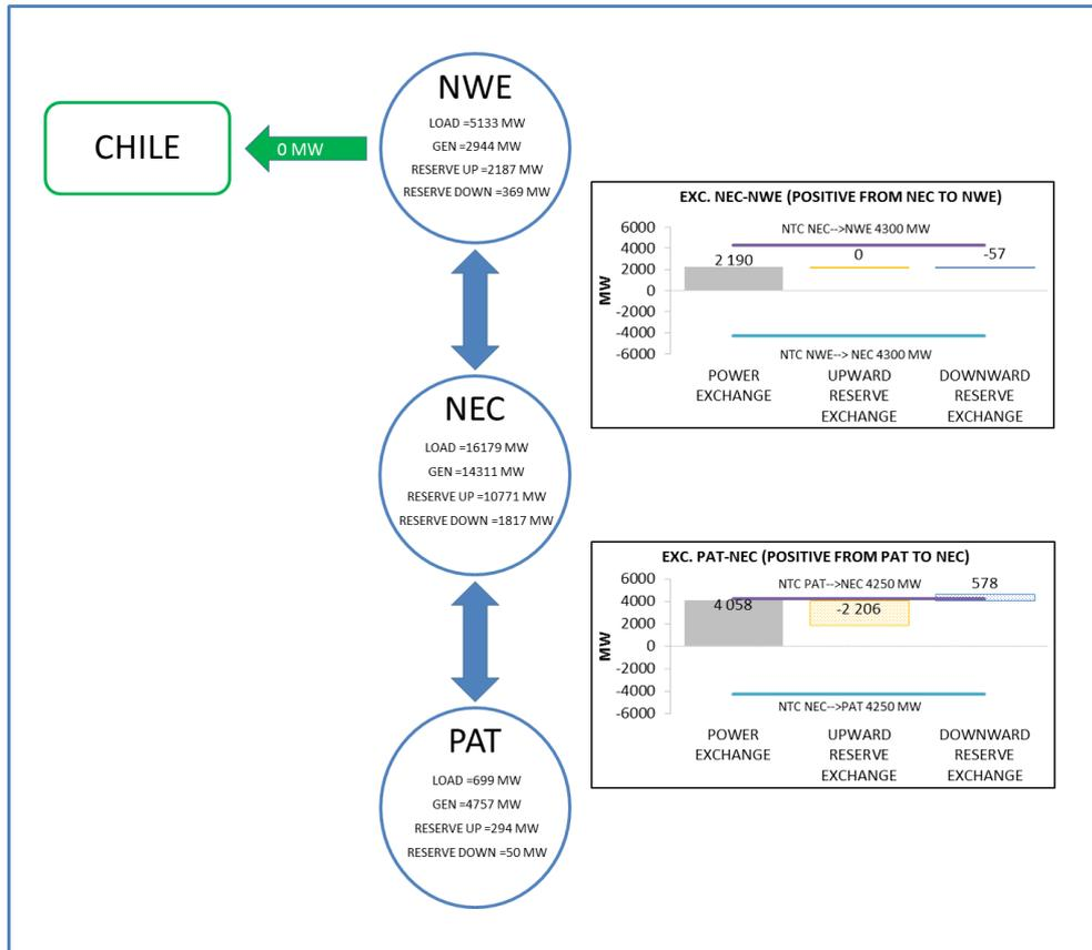
Figure 9 - Power and reserve exchanges between Argentinian areas - Low load and high VRES scenario, maximum wind installed capacity, no cross-border exchanges
