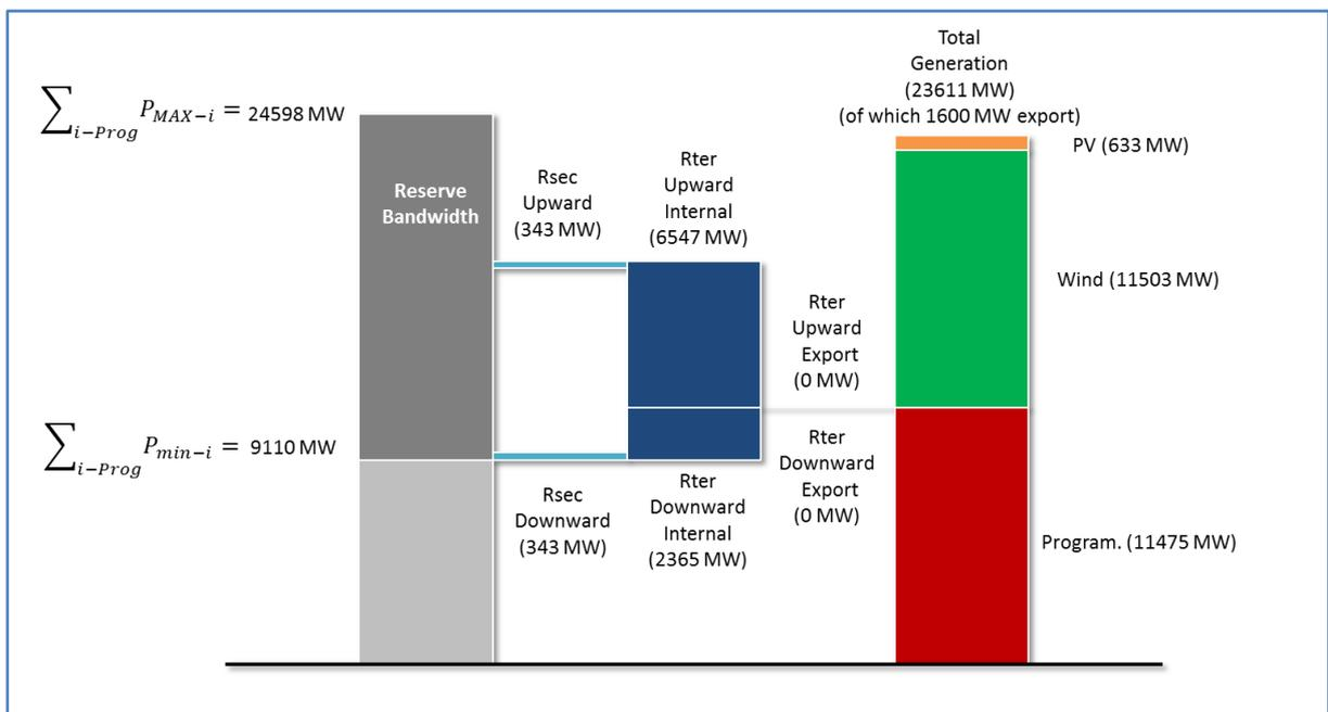
Figure 10 - Generation and reserve in Argentina - Low load and high VRES scenario, maximum wind installed capacity, maximum export
