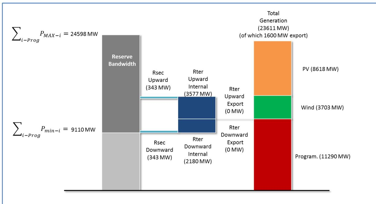
Figure 18 - Generation and reserve in Argentina - Low load and high VRES scenario, maximum PV installed capacity meeting wind target, maximum export
