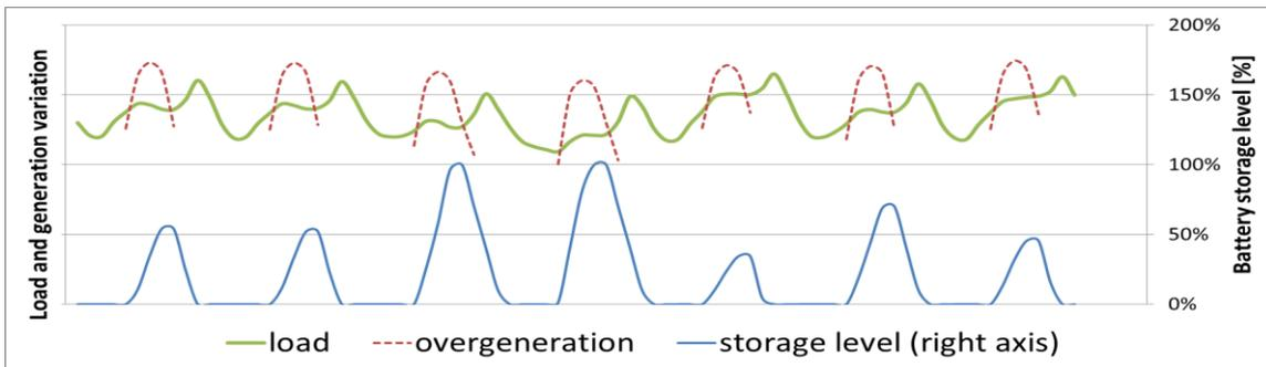
Figure 73 - Typical storage level cycles when associated to PV generation
