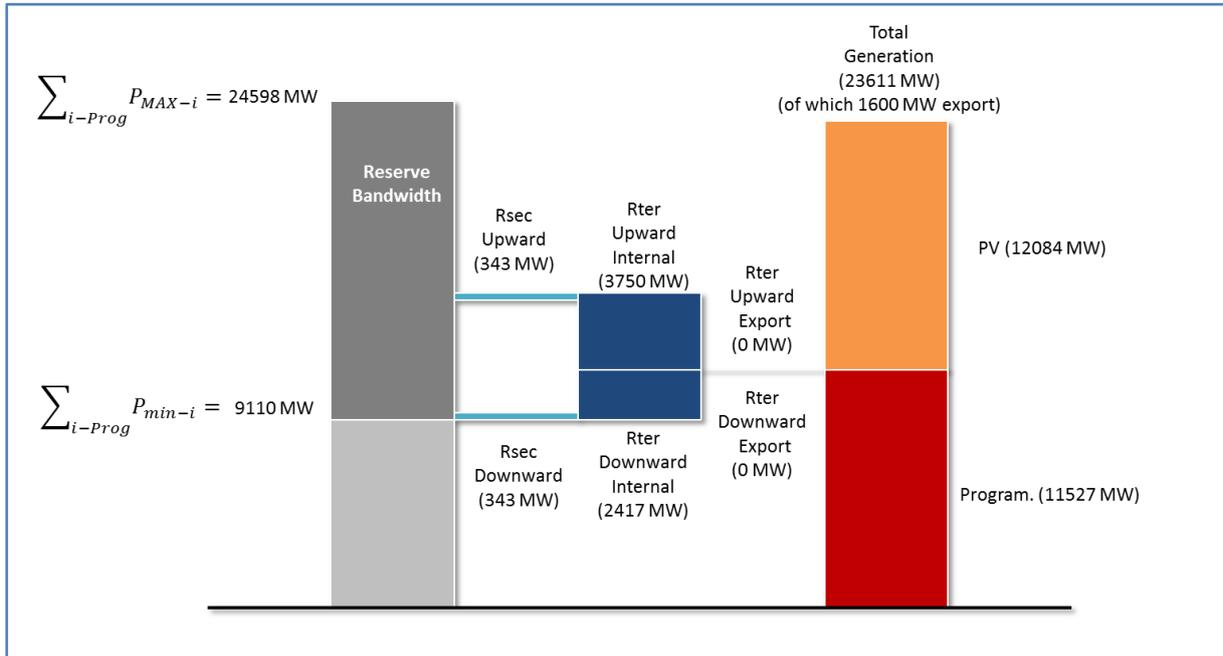
Figure 22 - Generation and reserve in Argentina - Low load and high VRES scenario, maximum PV installed capacity, maximum export
