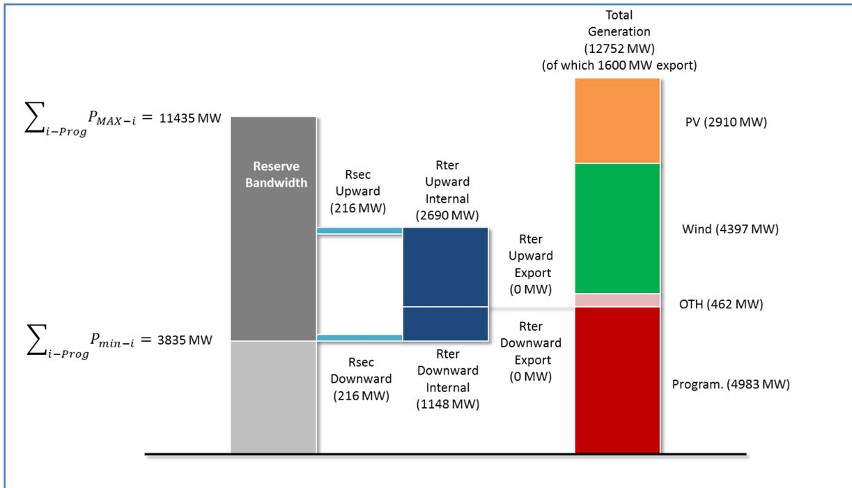
Figure 32 - Generation and reserve in Chile- Low load and high VRES scenario, maximum wind installed capacity meeting PV target, maximum export
