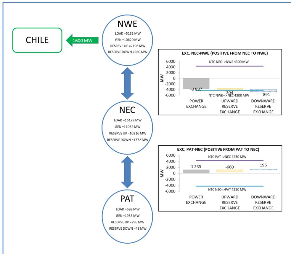
**Figure 19 - Power and reserve exchanges between Argentinian areas - Low load and high VRES scenario, maximum PV installed capacity meeting wind target, maximum export**
