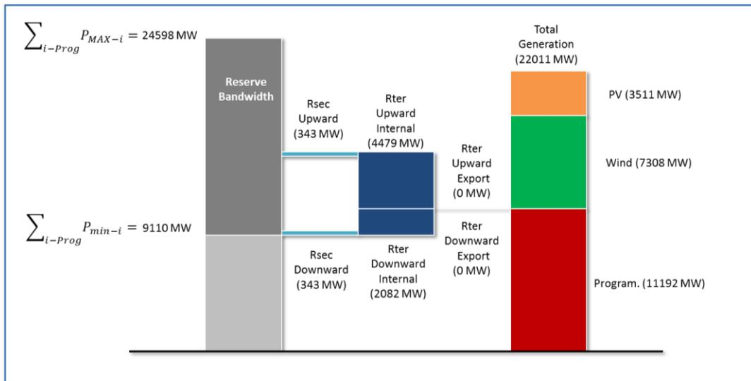
Figure 12 - Generation and reserve in Argentina - Low load and high VRES scenario, maximum wind installed capacity meeting PV target, no cross-border exchanges
