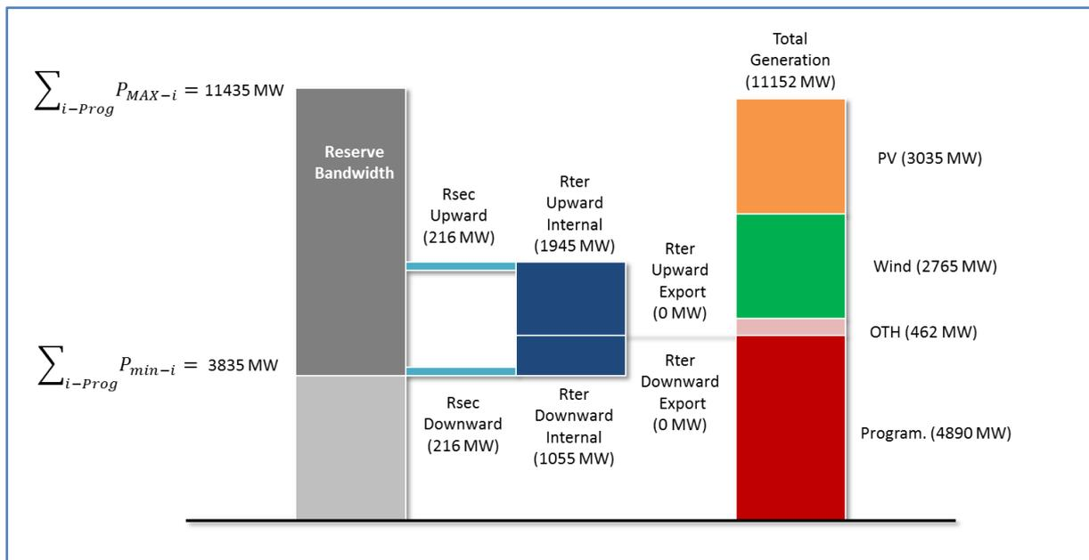
Figure 34 - Generation and reserve in Chile - Low load and high VRES scenario, maximum PV installed capacity meeting wind target, no cross-border exchanges
