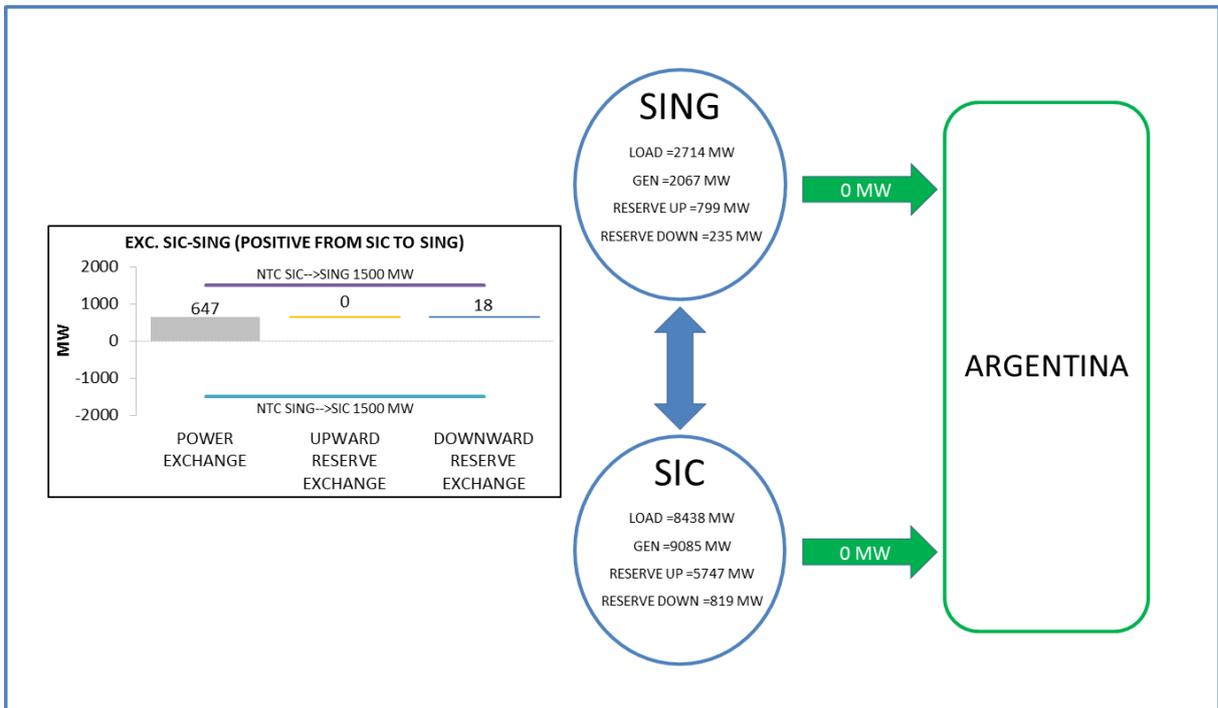
Figure 31 - Power and reserve exchanges between Chilean areas - Low load and high VRES scenario, maximum wind installed capacity meeting PV target, no cross-border exchanges
