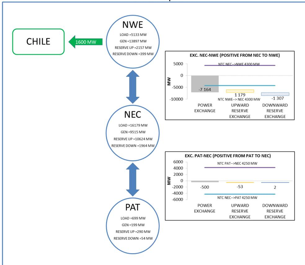
Figure 23 - Power and reserve exchanges between Argentinian areas - Low load and high VRES scenario, maximum PV installed capacity, maximum export
