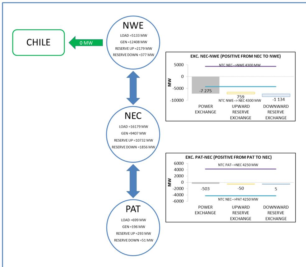
Figure 21 - Power and reserve exchanges between Argentinian areas - Low load and high VRES scenario, maximum PV installed capacity, no cross-border exchanges
