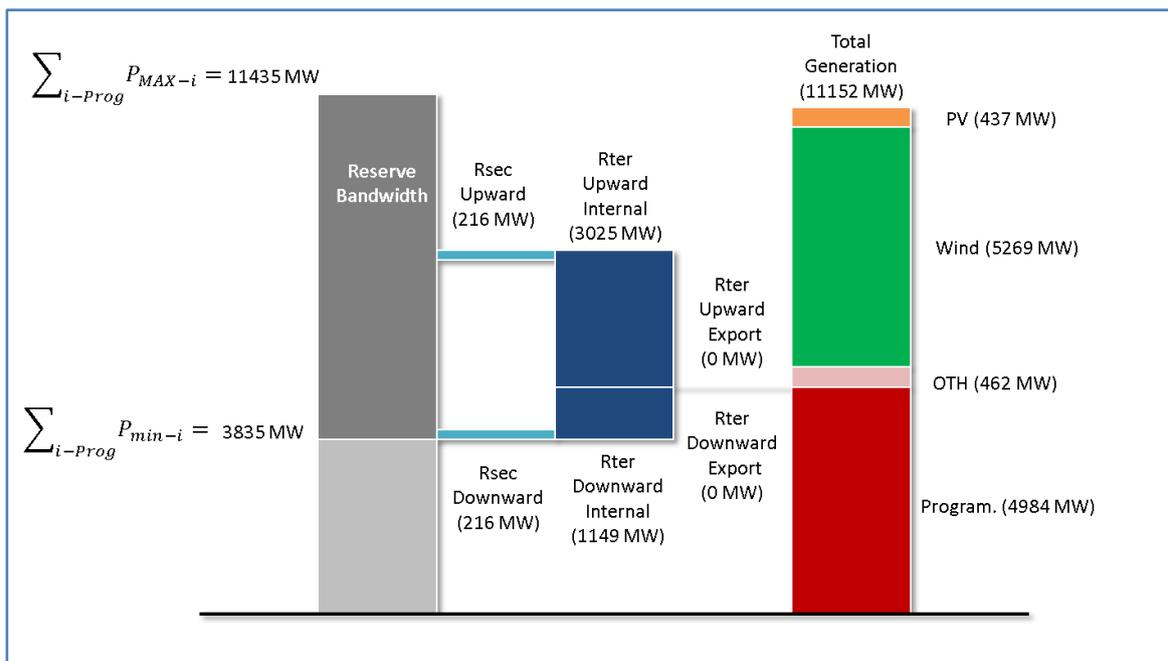
Figure 26 - Generation and reserve in Chile- Low load and high VRES scenario, maximum wind installed capacity, no cross-border exchanges
