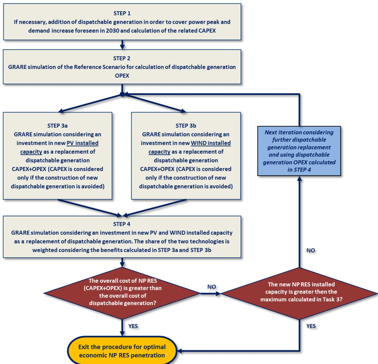
Figure 43 - Procedure for the calculation of the optimal economic VRES penetration
