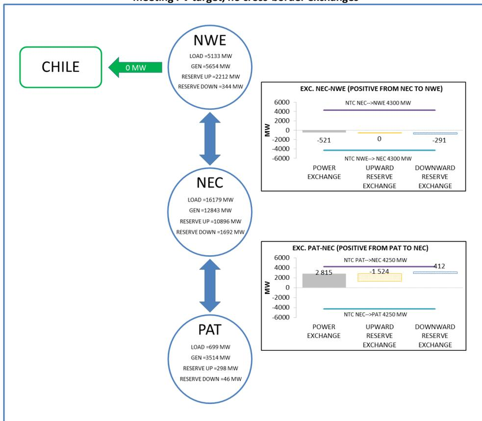
Figure 13 - Power and reserve exchanges between Argentinian areas - Low load and high VRES scenario, maximum wind installed capacity meeting PV target, no cross-border exchanges
