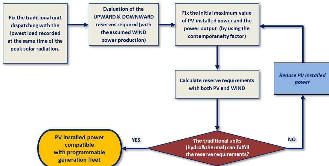
Figure 3 - iterative calculation of max installation of PV once assumed a fixed value of Wind
