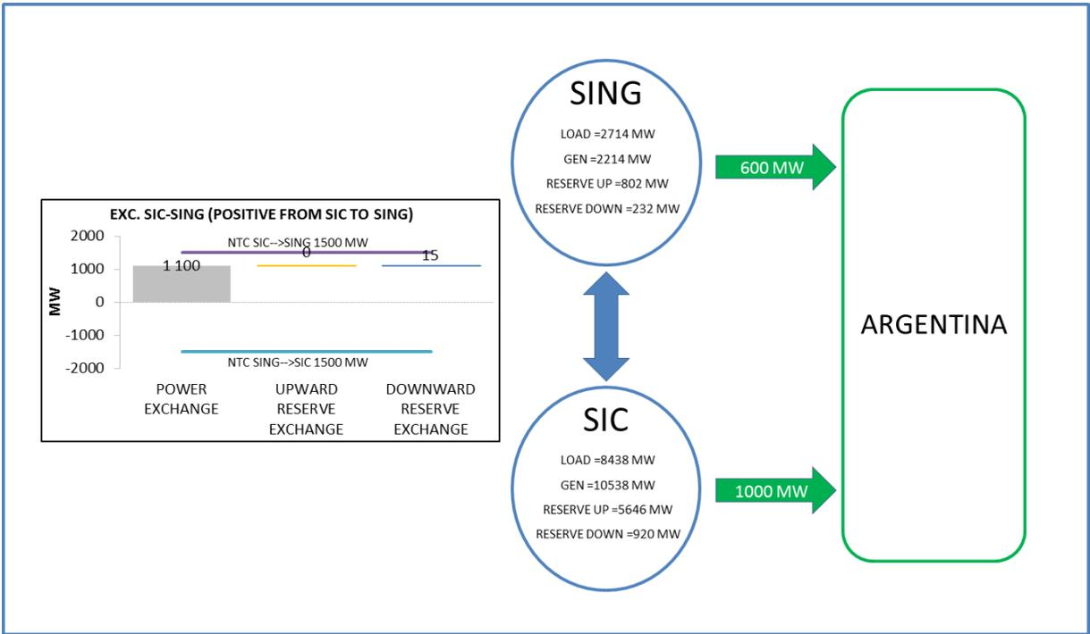
Figure 37 - Power and reserve exchanges between Chilean areas - Low load and high VRES scenario, maximum PV installed capacity meeting wind target, maximum export
