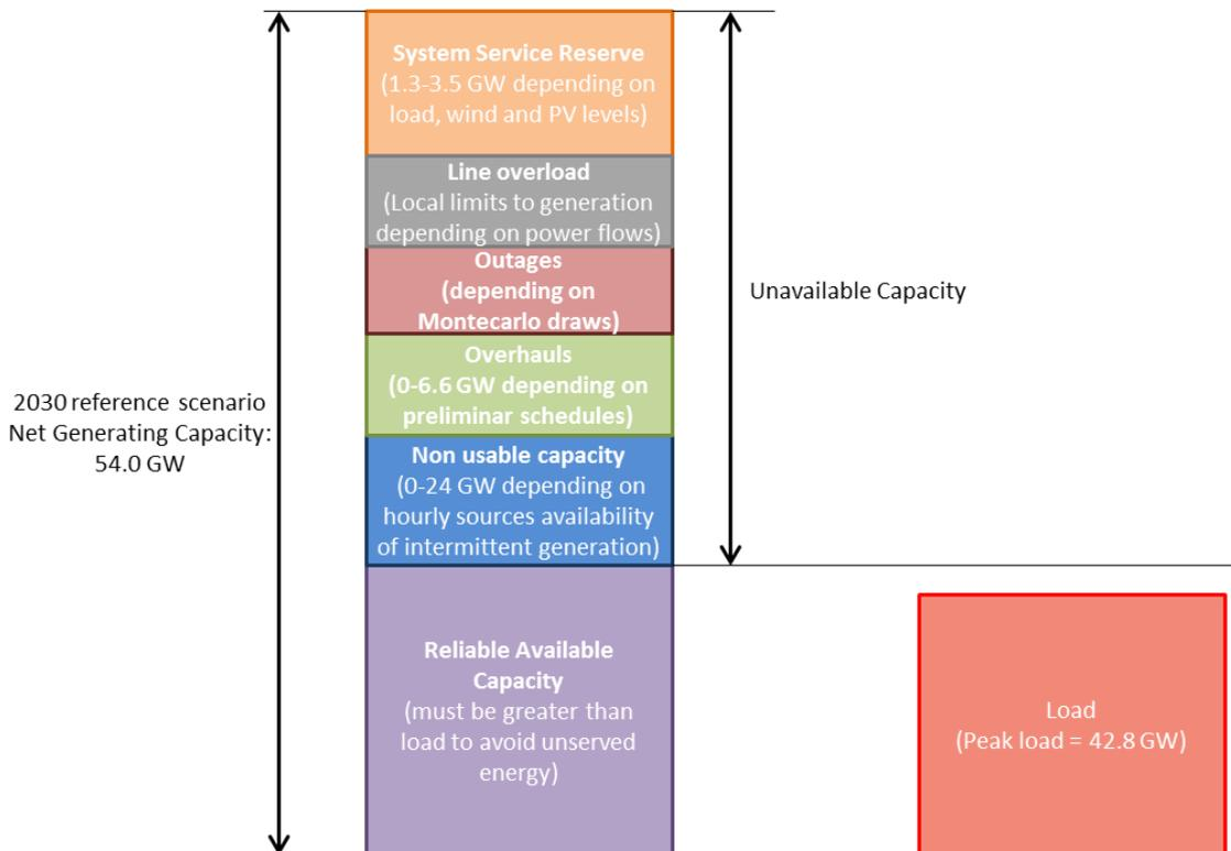
Figure 45 - Generation capacity reduction during operation in Argentina
