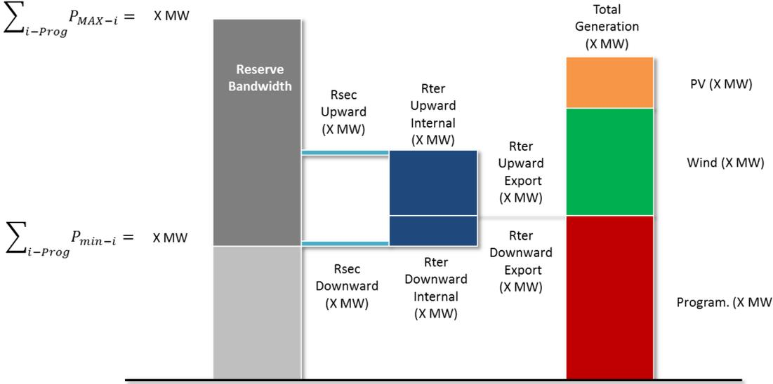
Figure 5 - Example of presentation of the upper bound limit definition for VRES installed capacity
