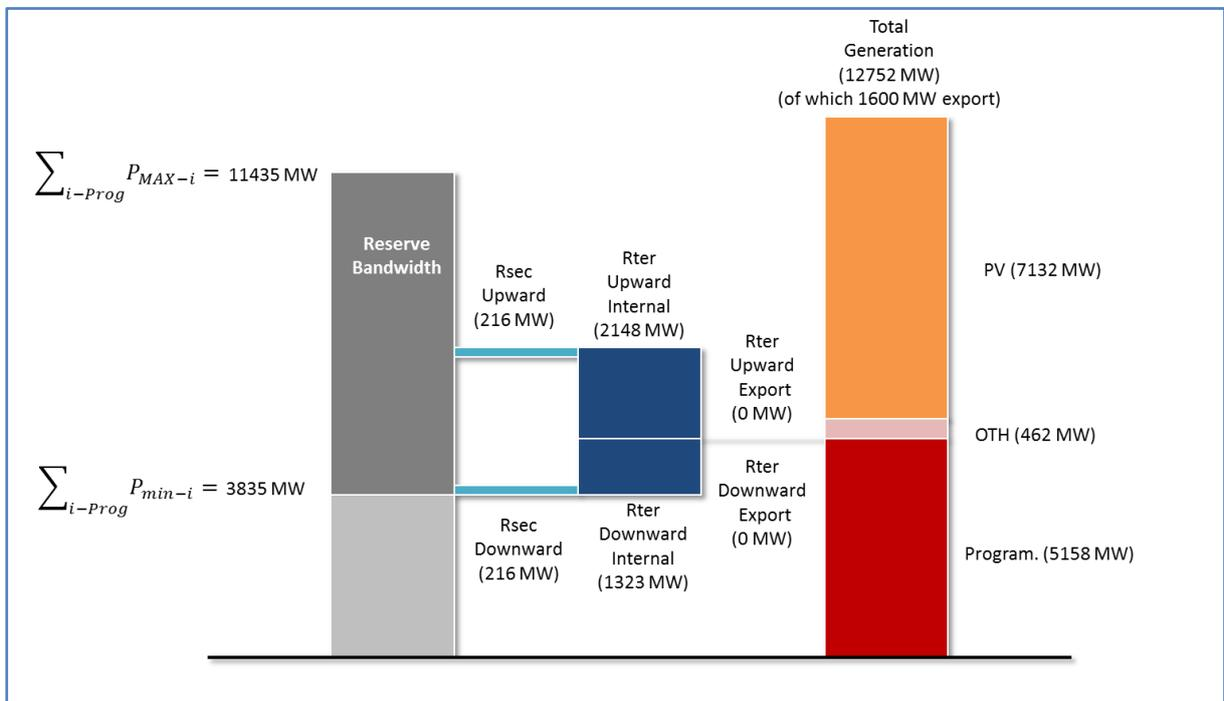
Figure 40 - Generation and reserve in Chile - Low load and high VRES scenario, maximum PV installed capacity, maximum export
