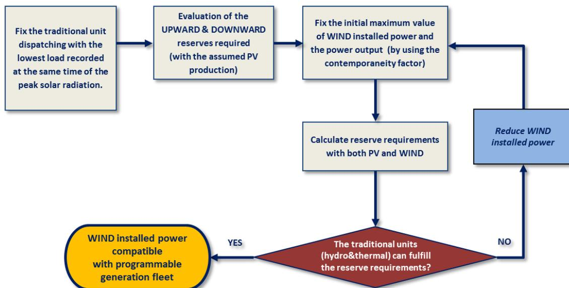
Figure 4 - iterative calculation of max installation of WIND once assumed a fixed value of PV
