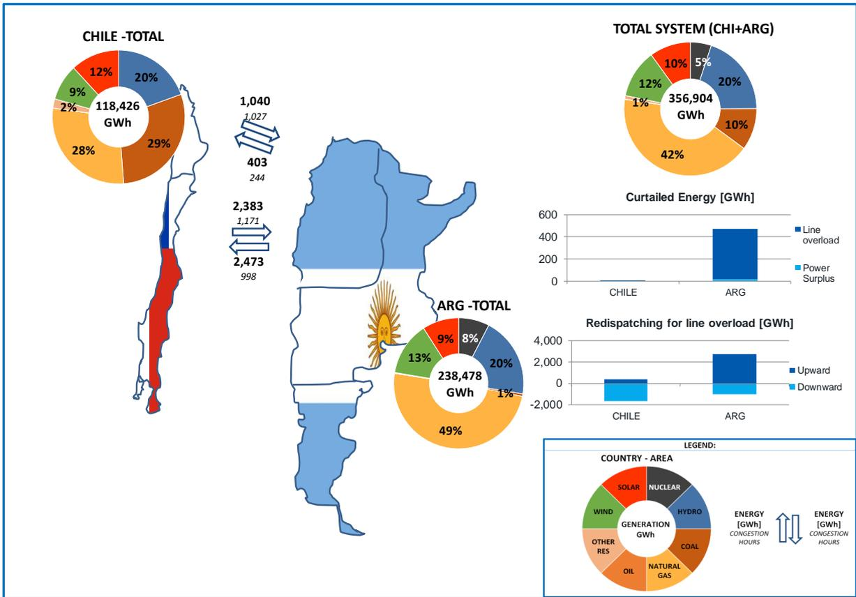
Figure 61 - Total production and energy exchanges —interconnected optimal scenario
