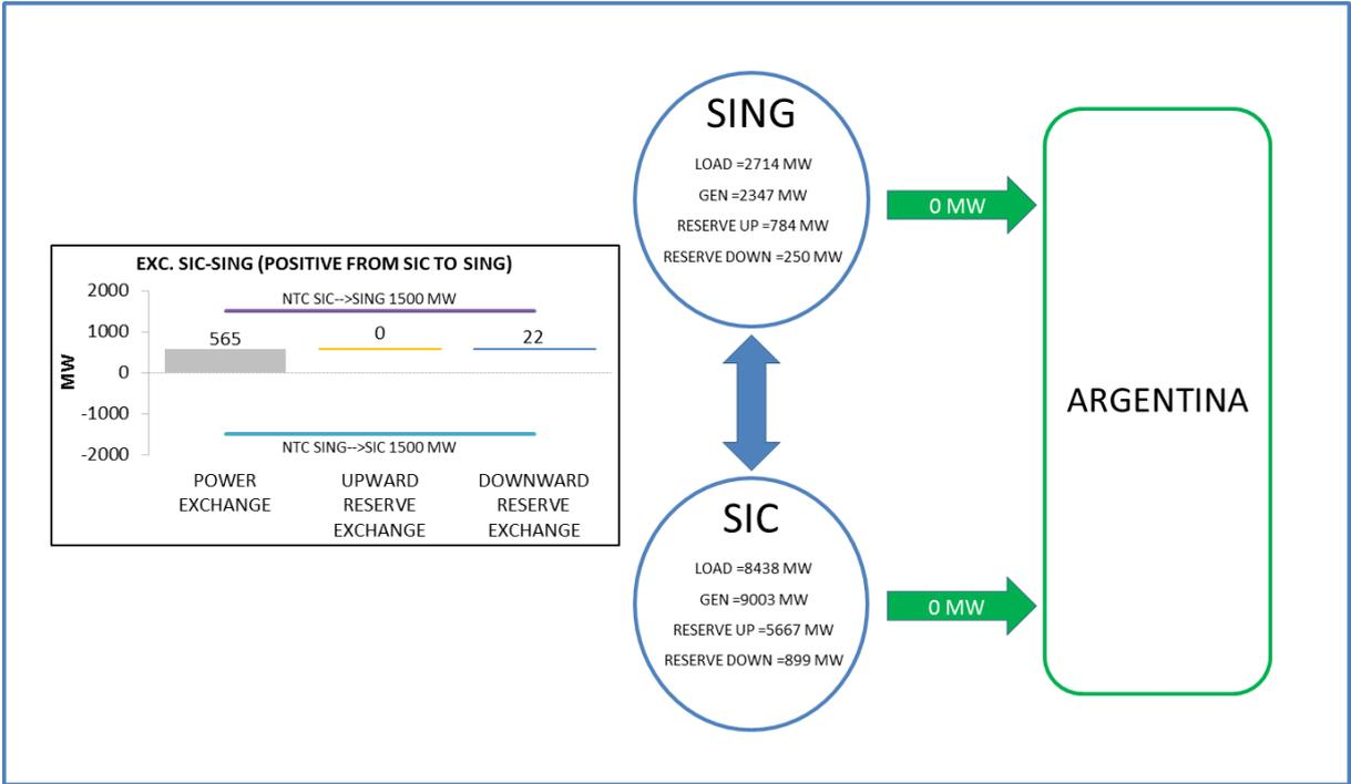
Figure 27 - Power and reserve exchanges between Chilean areas - Low load and high VRES scenario, maximum wind installed capacity, no cross-border exchanges
