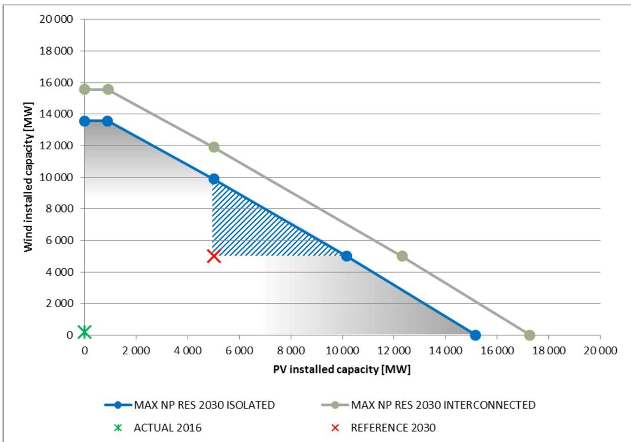
Figure 24 - resulting area of admissible PV /wind installed power fulfilling the system reserve requirements
