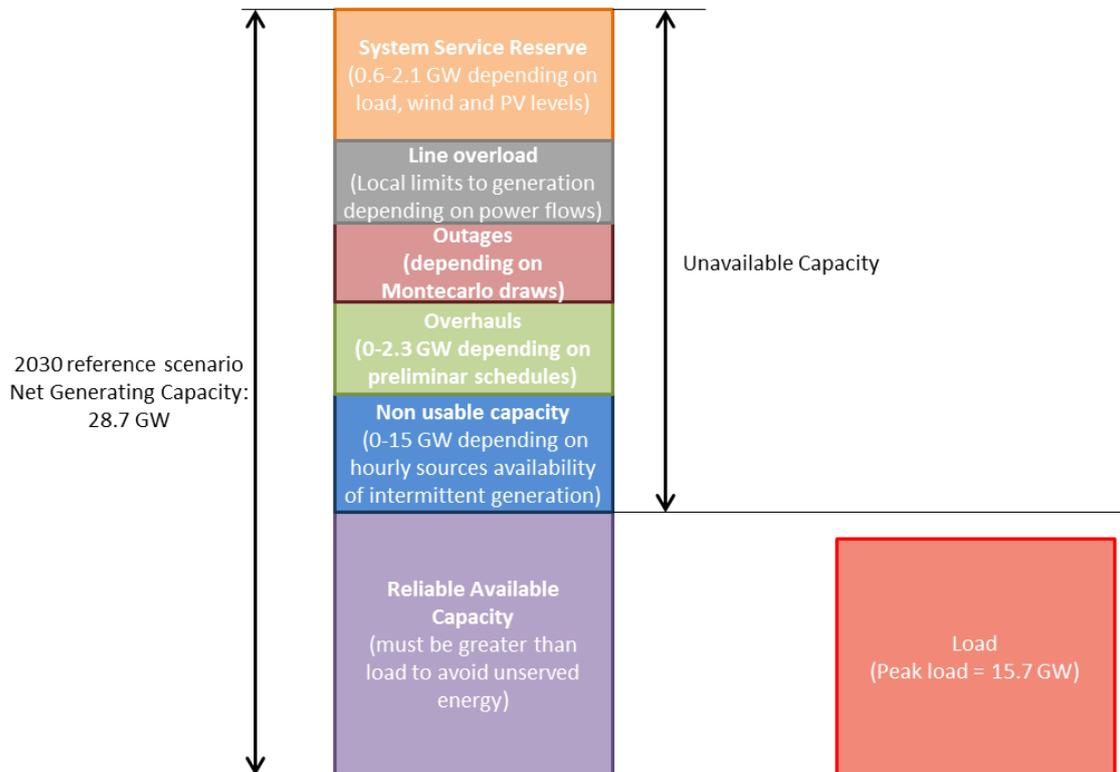
**Figure 47 - Generation capacity reduction during operation in Chile**
