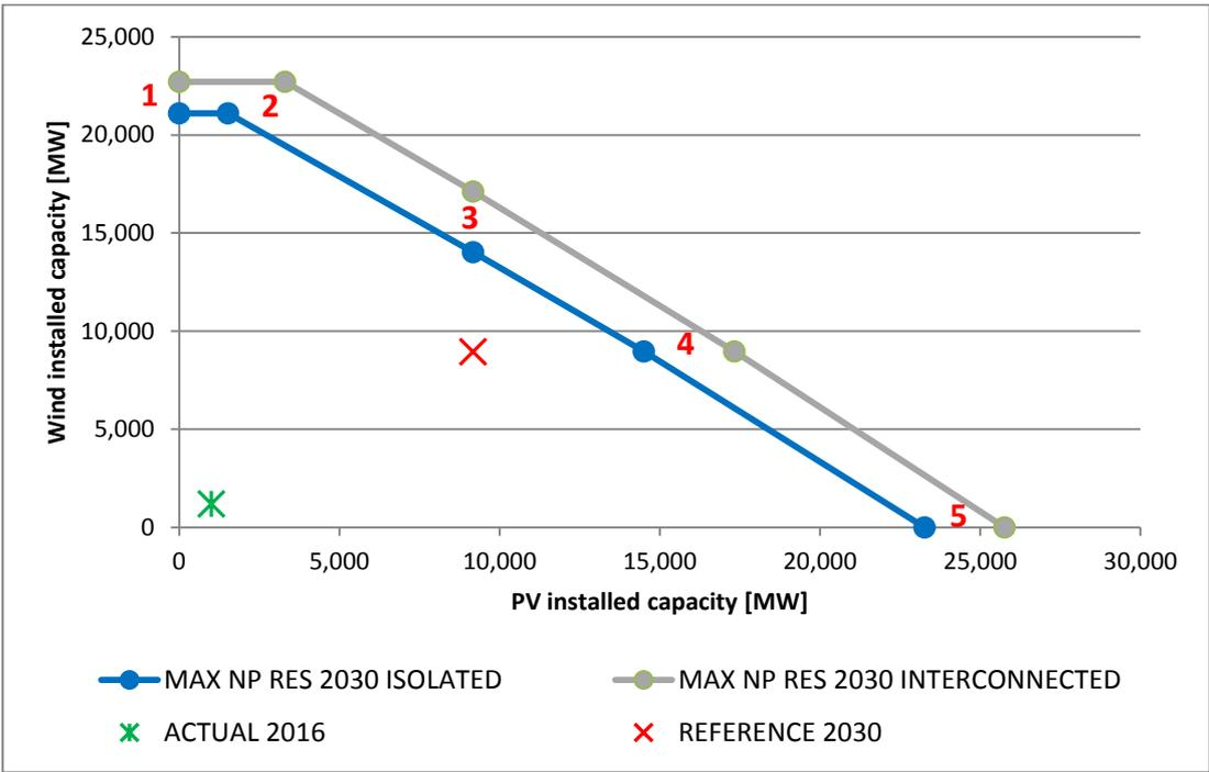
Figure 42 - VRES installed capacity limits due to system operation constraints in Chilean and Argentinian interconnected system - 2030
