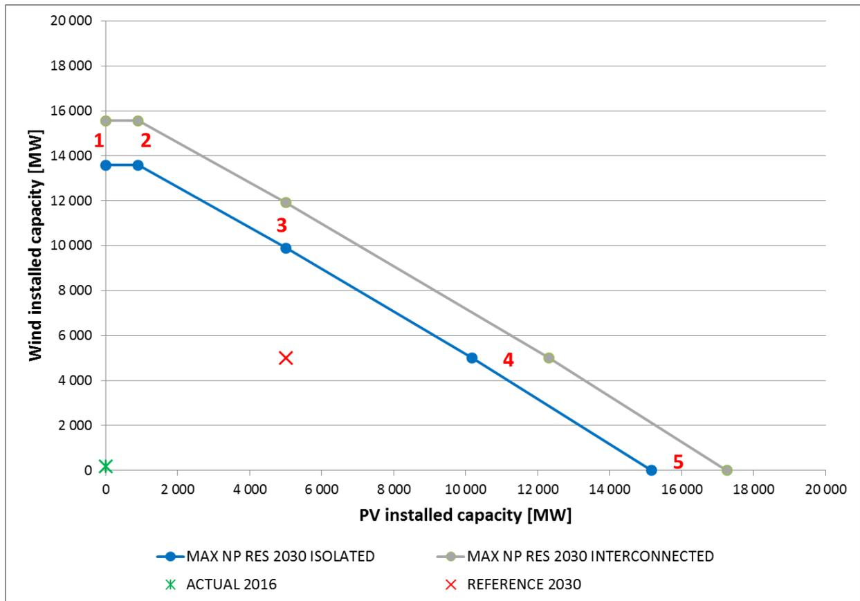
Figure 7 - VRES installed capacity limits due to system operation constraints in Argentina – 2030
