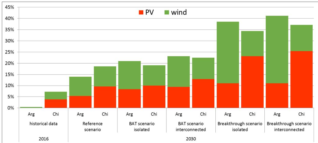
Figure 78 - Net load coverage by PV and wind plants in different scenarios
