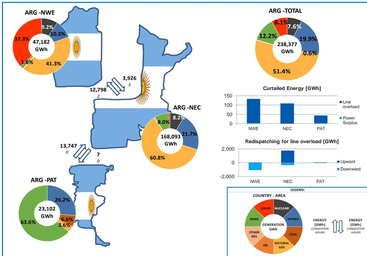
Figure 55 - Total production and energy exchanges – Argentinian scenario with relocation of some PV power plants from NWE to NEC
