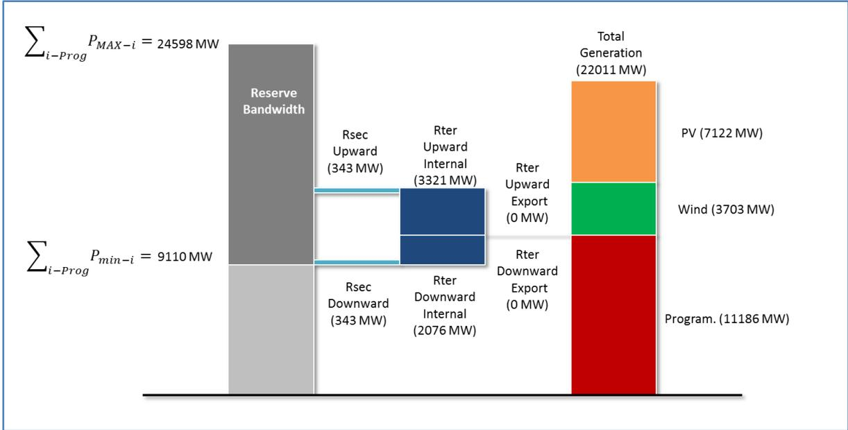
Figure 16 - Generation and reserve in Argentina - Low load and high VRES scenario, maximum PV installed capacity meeting wind target, no cross-border exchanges
