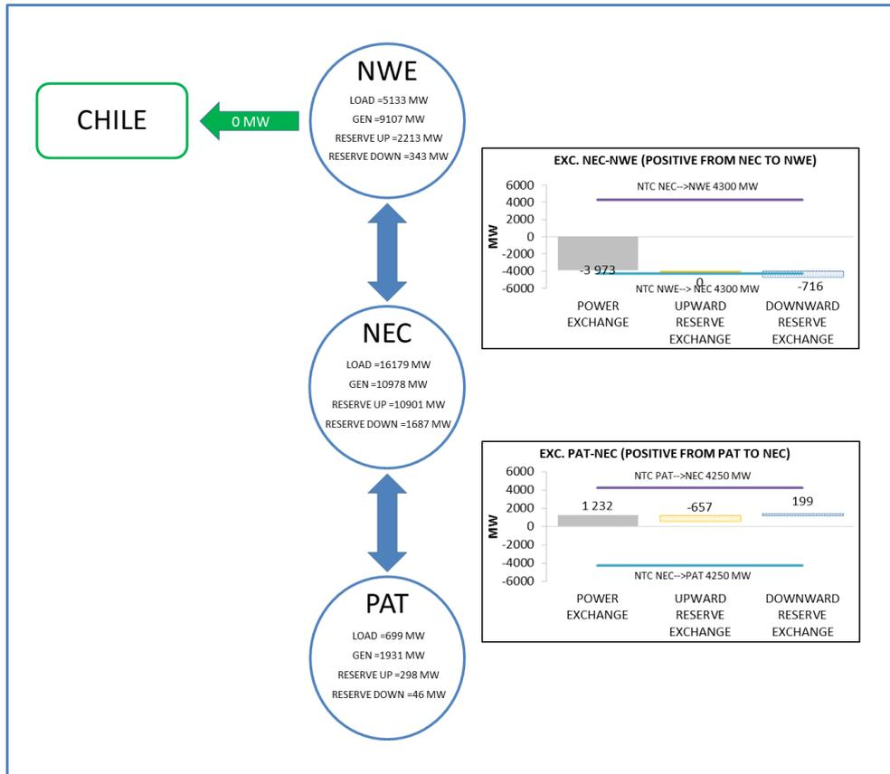
Figure 17 - Power and reserve exchanges between Argentinian areas - Low load and high VRES scenario, maximum PV installed capacity meeting wind target, no cross-border exchanges
