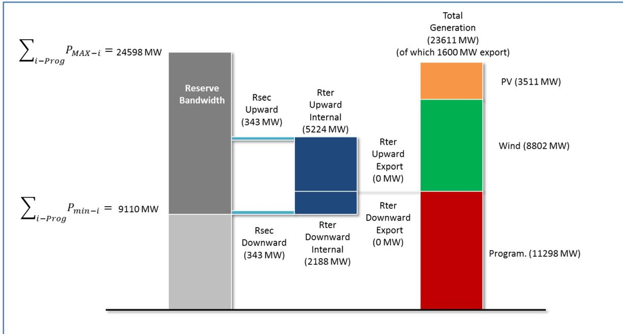
Figure 14 - Generation and reserve in Argentina - Low load and high VRES scenario, maximum wind installed capacity meeting PV target, maximum export
