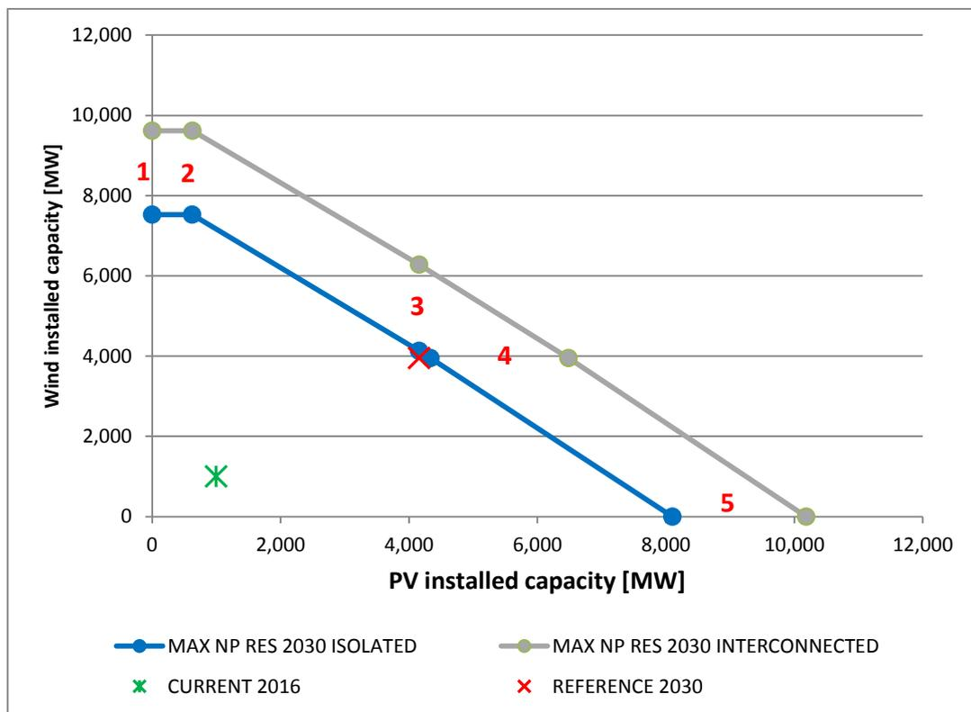
Figure 25 - VRES installed capacity limits due to system operation constraints in Chile - 2030
