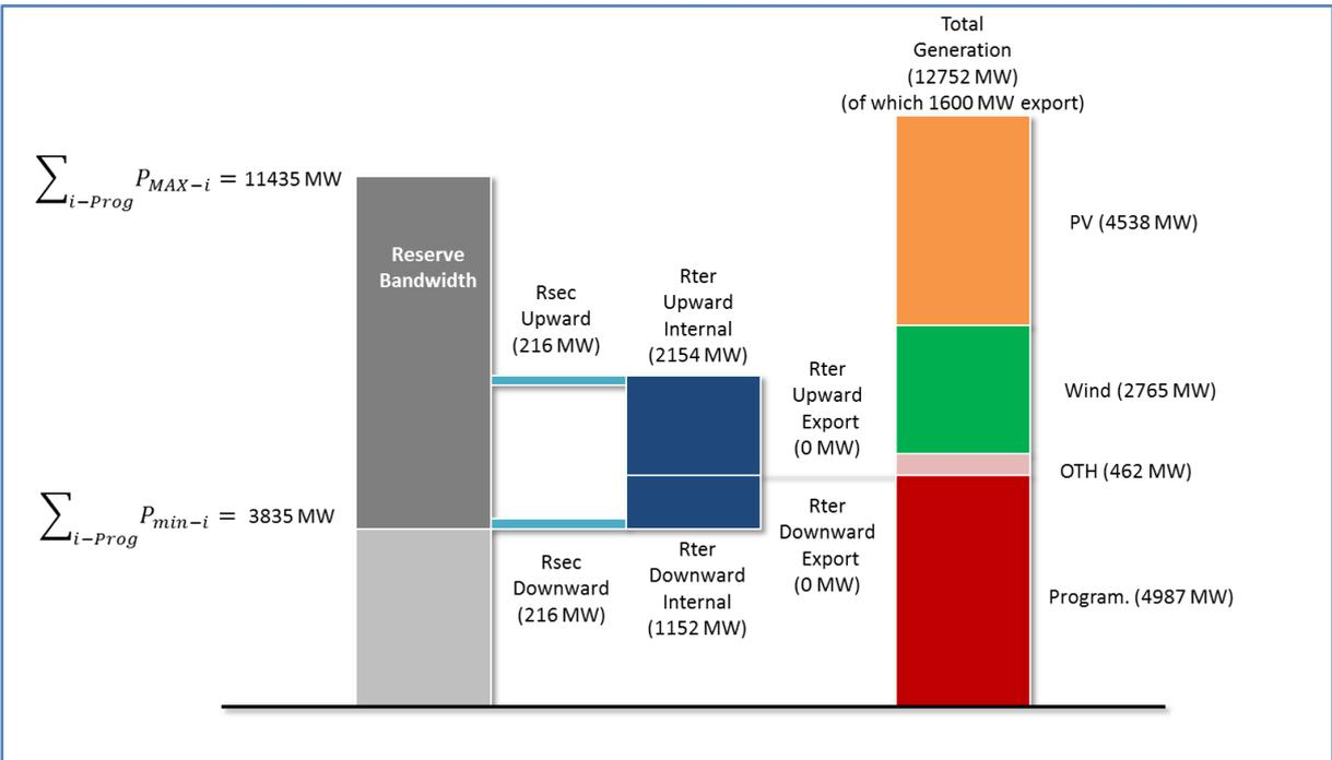
Figure 36- Generation and reserve in Chile - Low load and high VRES scenario, maximum PV installed capacity meeting wind target, maximum export
