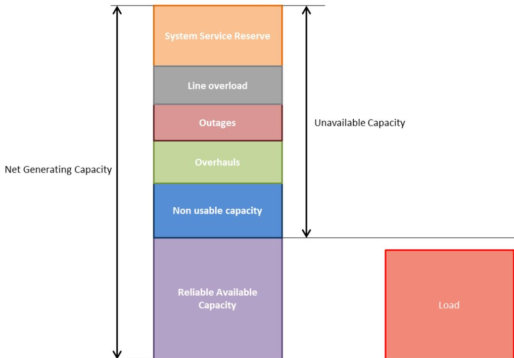
**Figure 44 - Overview of different causes of generation capacity reduction during operation**
