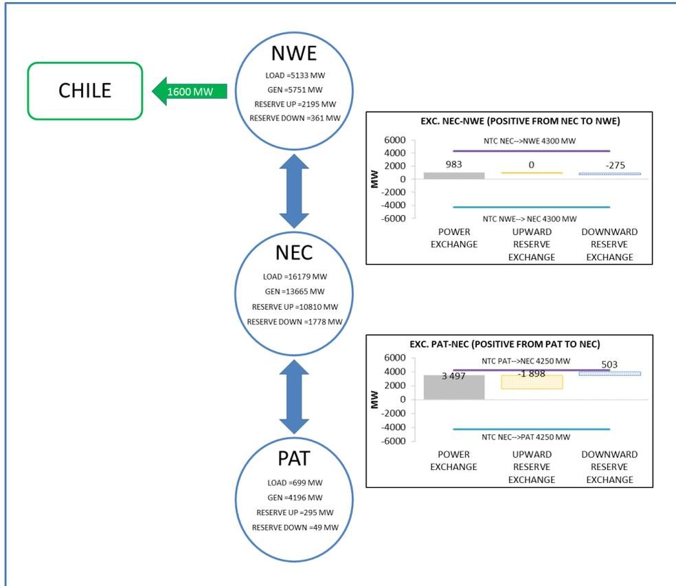
Figure 15 - Power and reserve exchanges between Argentinian areas - Low load and high VRES scenario, maximum wind installed capacity meeting PV target, maximum export
