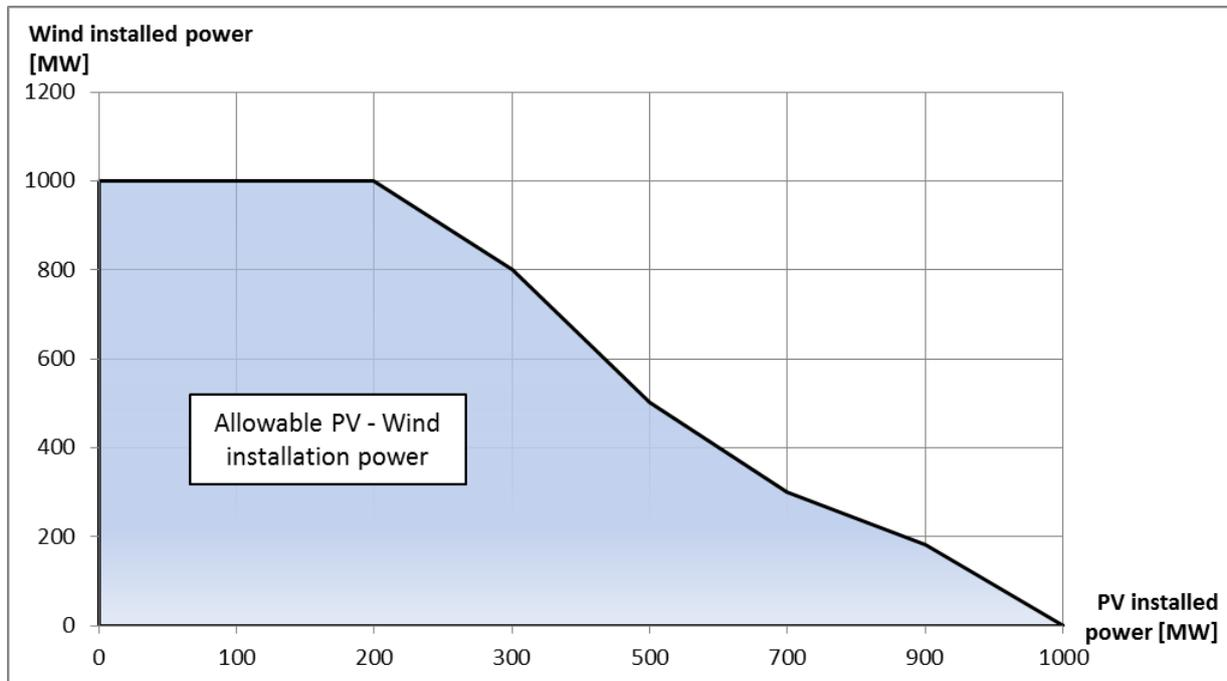
Figure 1 - Example of the allowable area on the PV/Wind installed power chart
