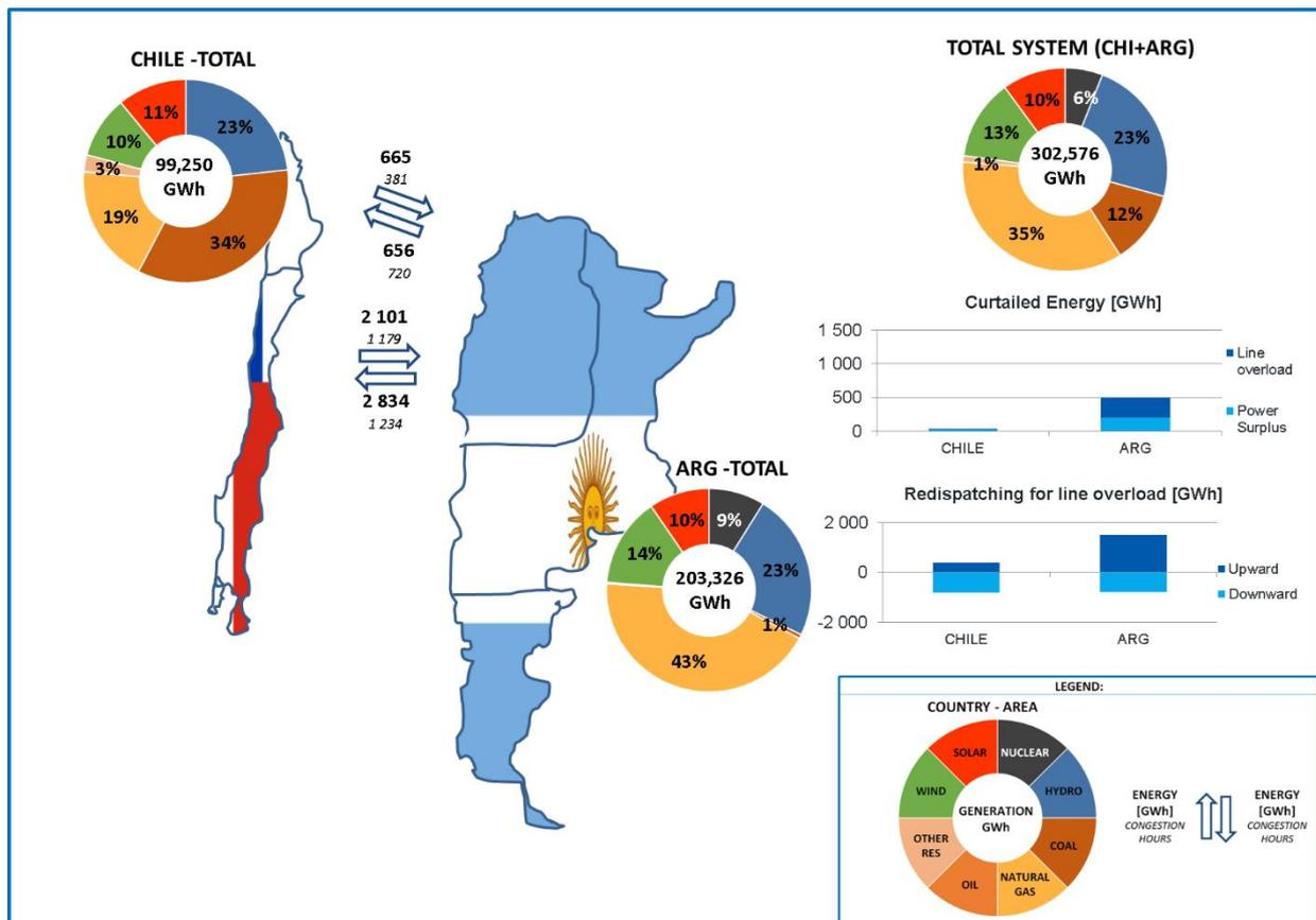
Figure 67 - Scenario V2a - Total production and energy exchanges
