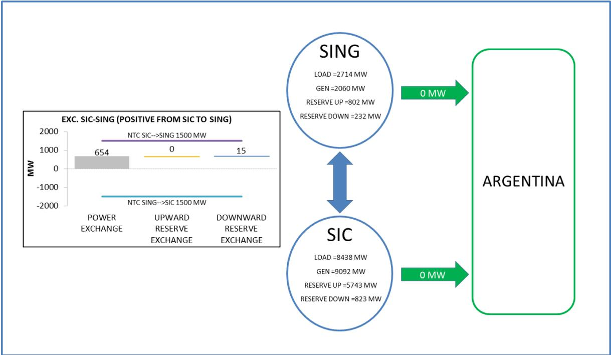
Figure 35 - Power and reserve exchanges between Chilean areas - Low load and high VRES scenario, maximum PV installed capacity meeting wind target, no cross-border exchanges
