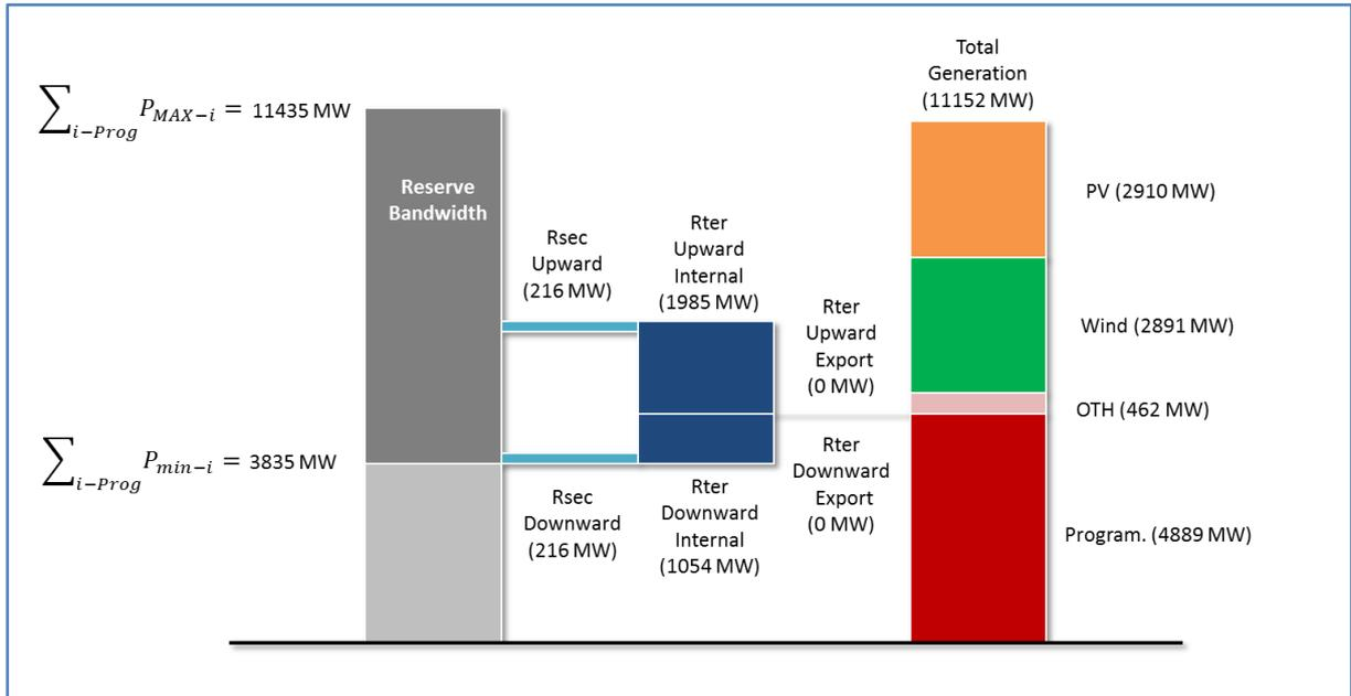
Figure 30 - Generation and reserve in Chile - Low load and high VRES scenario, maximum wind installed capacity meeting PV target, no cross-border exchanges
