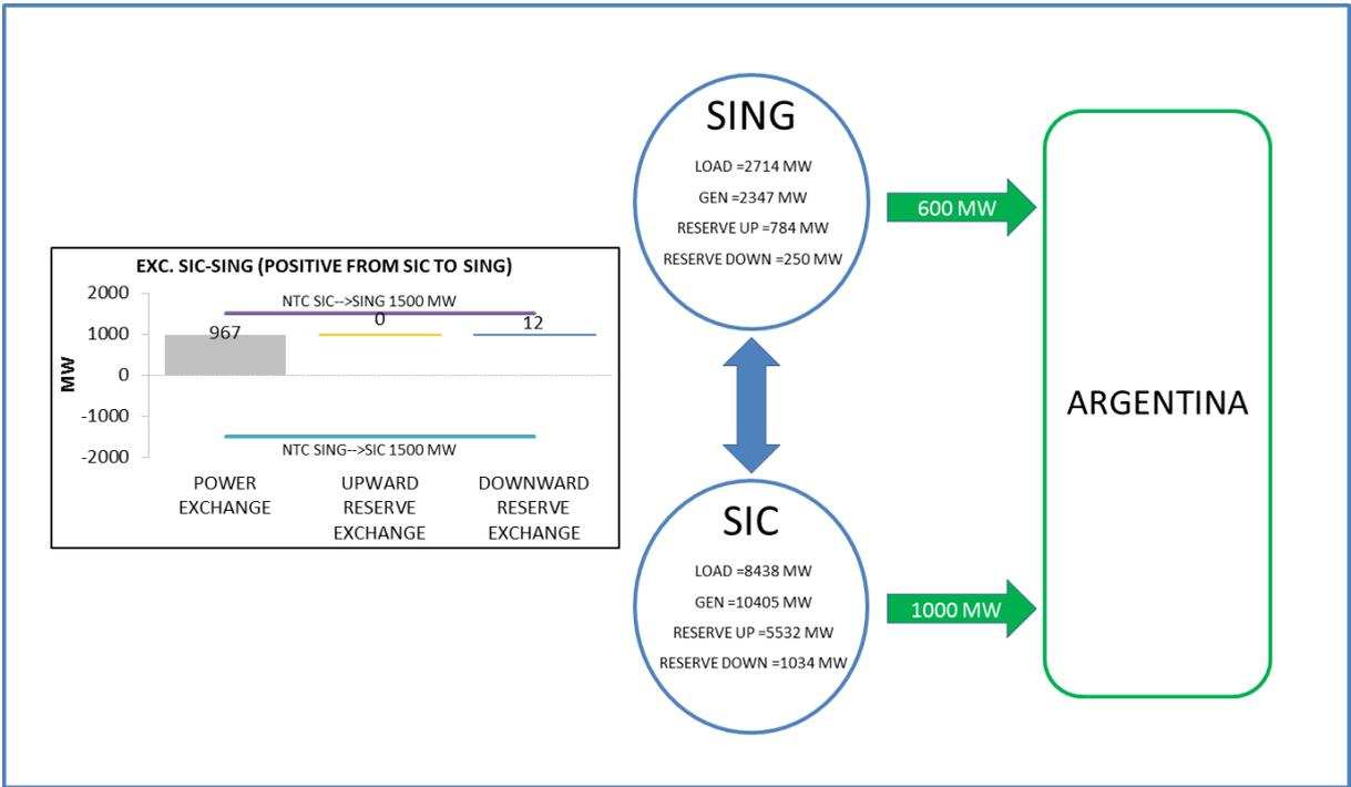
Figure 29 - Power and reserve exchanges between Chilean areas - Low load and high VRES scenario, maximum wind installed capacity, maximum export
