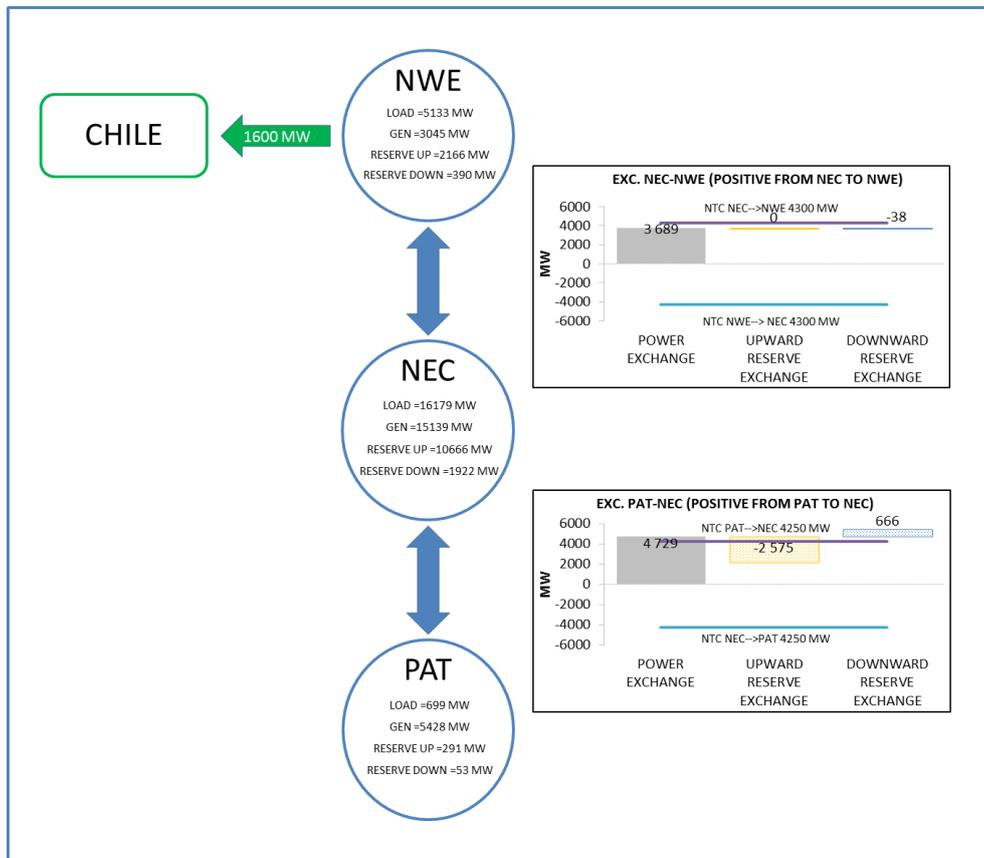
**Figure 11 - Power and reserve exchanges between Argentinian areas - Low load and high VRES scenario, maximum wind installed capacity, maximum export**
