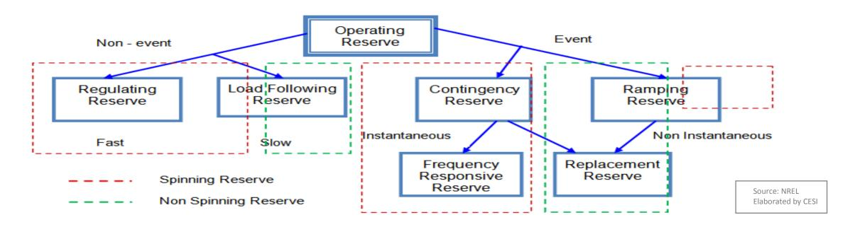
This study focuses <u>on the variation of requirement and cost relevant to spinning reserve</u> needed in electric power systems with high VRES penetration mainly for fast regulation and frequency control after contingencies
